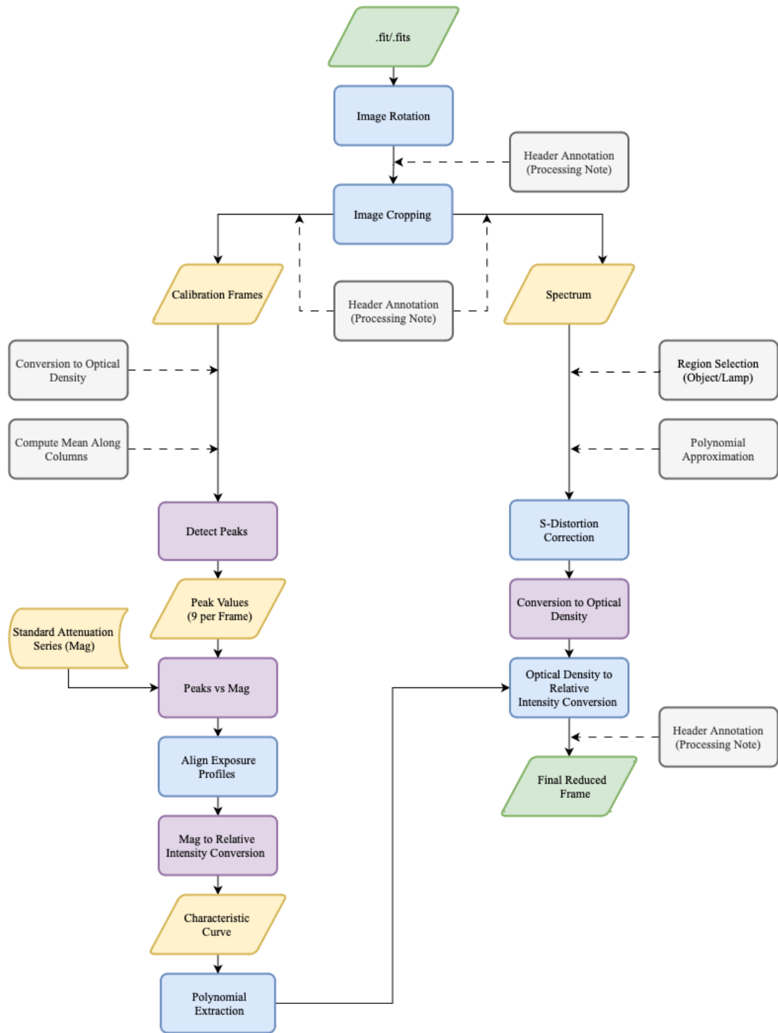
Figure 6.1: Flowchart illustrating the preprocessing of archival spectroscopic data. Green — input and output files; yellow — intermediate results; blue — automated processes; purple — manual processes; grey — background operations.
